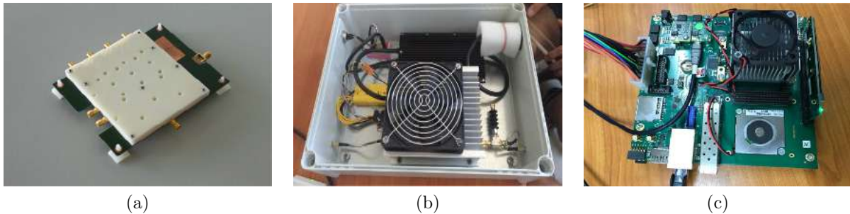
Figure 3. SAR Payload - (a) front-end, (b) power amplifier, (c) embedded digital radar processor.
