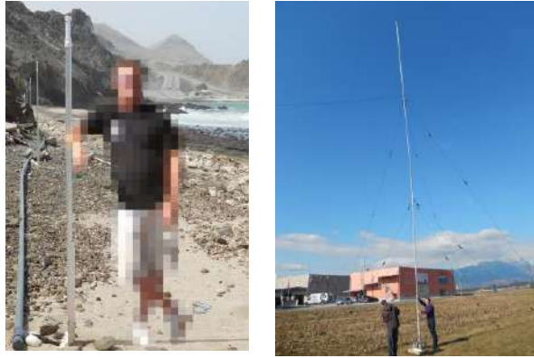
Fig. 4: Two different kinds of antennas. Left: active receive antenna with low visual impact, right: passive transmit antenna.
