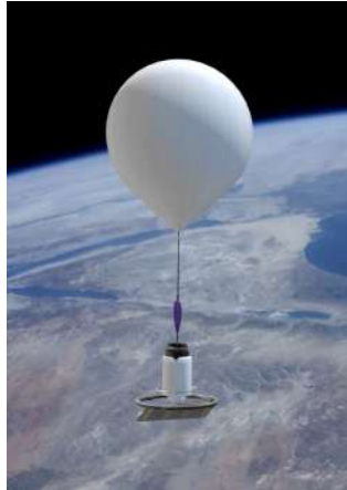
Figure 1. Illustration of the BALSAR system. Note that the radome is not drawn in order to show the antennas.
