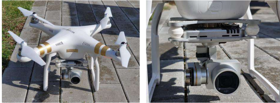
Figure 1: On the left hand side the Phantom3 Professional from DJI on the right hand side the Brushless gimbal with the 4K video camera mounted below the aircraft.
