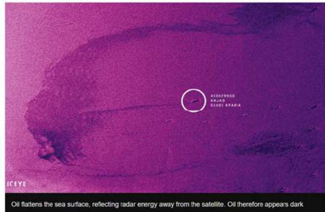
Figure 1. Radar imagery of possible oil transshipment; and radar intelligence on a resulting oil spill from a Saudi tanker
