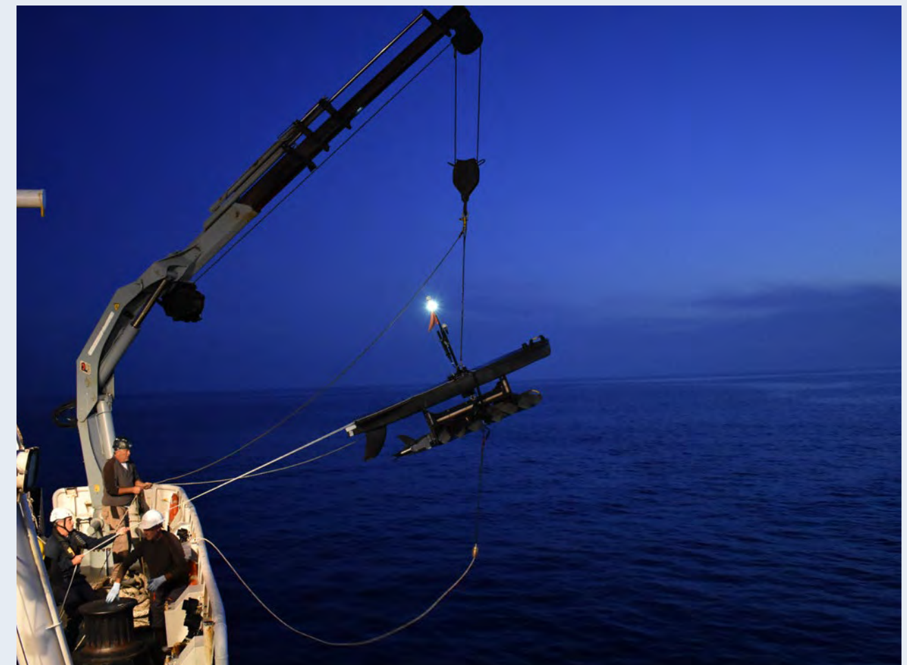
CMRE technicians deploy a wave glider during the REP-MUS'19 exercise in Portugal as part of underwater communications and networking experiments.
