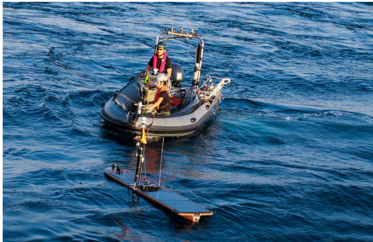
CMRE staff recover a wave glider during the Recognized Environmental Picture, Atlantic 2018 (REP18-Atlantic) exercise.
