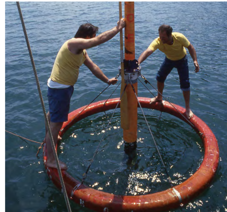
Above: c. 1970s. Crews deploy a meteo-oceanographic spar buoy from the Manning . Photos by: Federico de Strobel.
