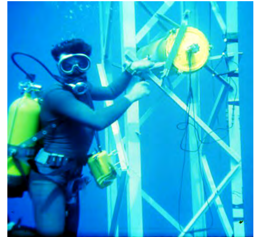
Above: c. 1960s. A meteo-oceanographic spar buoy being equipped with sensors by Centre divers. Photos by: Federico de Strobel.
