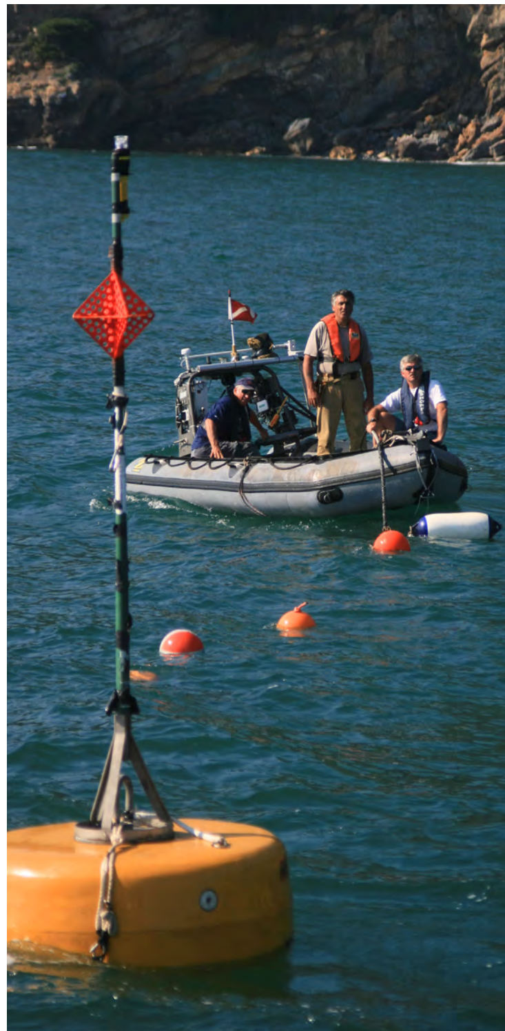
Left Page: 2007. Tomas Folegot, Domenico Galletti and Andrea Cavanna test a monitoring system made from thermistor chains to measure the water temperature profile.
