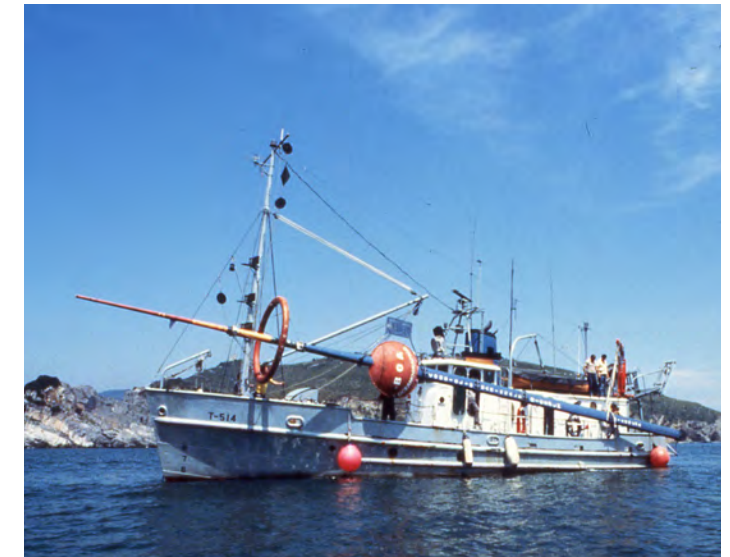
Above: c. 1970s. Crews deploy a meteo-oceanographic spar buoy from the Manning . Photos by: Federico de Strobel.
