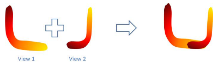
Fig. 2. Schematic concept of registration of two SAS snippets with data acquired at a 90 degrees difference angle.
