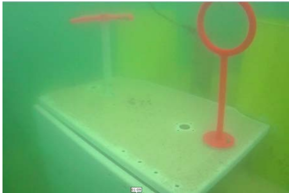
Fig. 6. The console containing the object to be manipulated: an orange valve and the stick-ring structure. Low visibility conditions were present during the competitions in the CMRE basin area.
