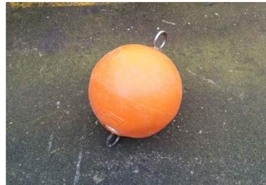
Fig. 4. An OPI. The outer diameter of the sphere is 30 cm. The buoys were moored at 1.5 m from the bottom.
