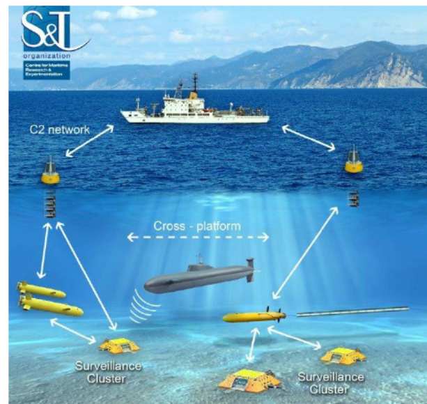
Fig. 1. Generic heterogeneous UW communications concept comprising manned and unmanned, static and mobile platforms interconnecting the UW world with command and control networks
