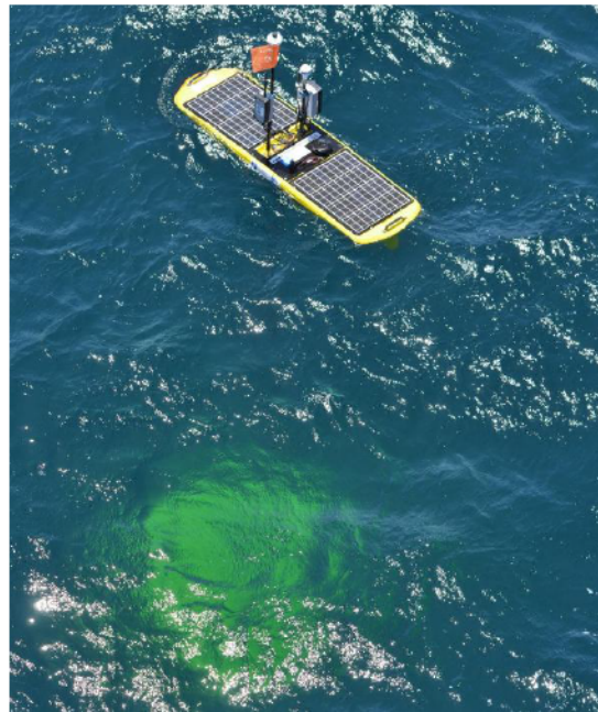
Fig. 7. The LRI Waveglider vehicle was modified by CMRE to have a "backseat" driving computer. It is currently used as a mobile, self-relocatable gateway.
