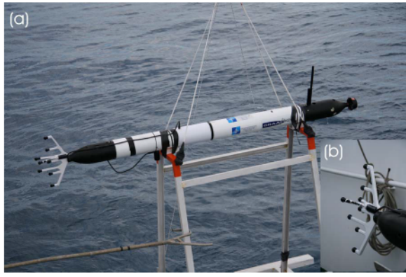
Fig. 4. The eFOLAGA AUV with nose array (a) and the array itself (b) ready for deployment. The eFOLAGA is here shown fixed on a purposely designed frame to be moored on the bottom.
