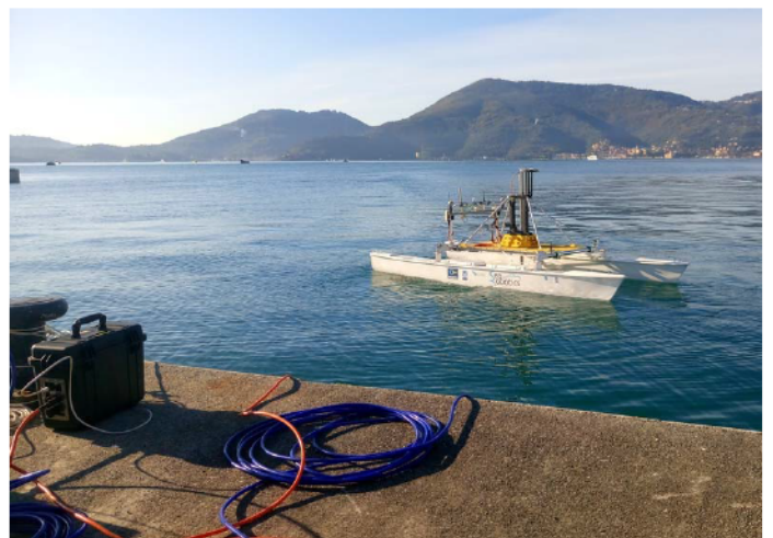
Fig. 3. The USV Gulliver used as a node of the underwater acoustic network as well as one portable node in the bottom-left corner. The Gulliver had the id=10 and is the target of localisation in our paper.
