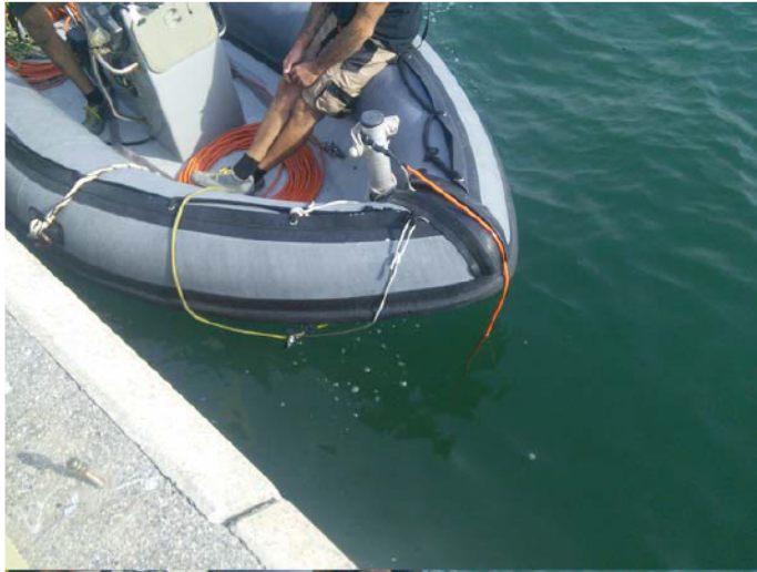
Fig. 4. Acoustic modem deployed over the bow of the supporting rubber boat.
