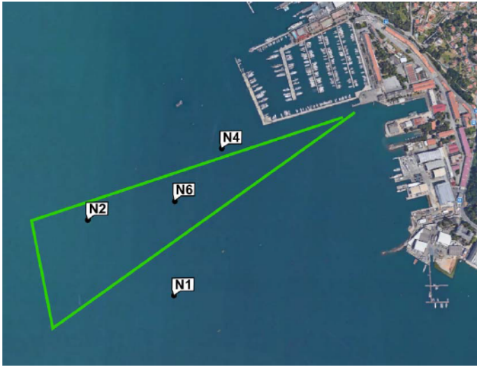
Fig. 3. Littoral Ocean Observatory Network (LOON) modem deployment (N1,N2,N4,N6). The picture also shows in green the desired trajectory for the mobile node on September 29 th .
