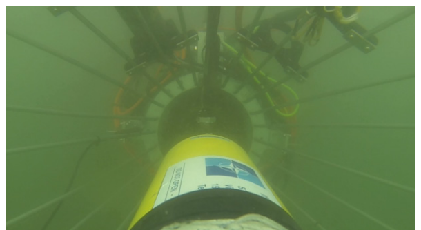
AUV docking underwater for battery recharging and data exchange in CMRE harbour during a two-week continuous demonstration in November 2017
