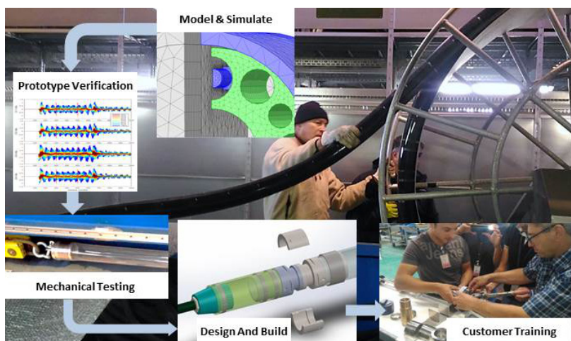
Main photo: winding the array onto a drum, ready for delivery. Insets: show some of the key phases in the design and realisation of the LDS array: FEM simulation; acoustic prototype evaluation; tension and vibration testing; mechanical design and customer training.
