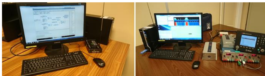
Figure 1. Two computers, Gnuradio, Balduzzi (improved), SDRsharp, AISMon, openCPN, Matlab, SAAB R4, SAAB R5 secured, HackRF, VHF USB dongle, and additional advanced SDR equipment for lab experiments. Also includes a mobile platform based on a laptop containing all falsification and detection features allowing for external experiments.
