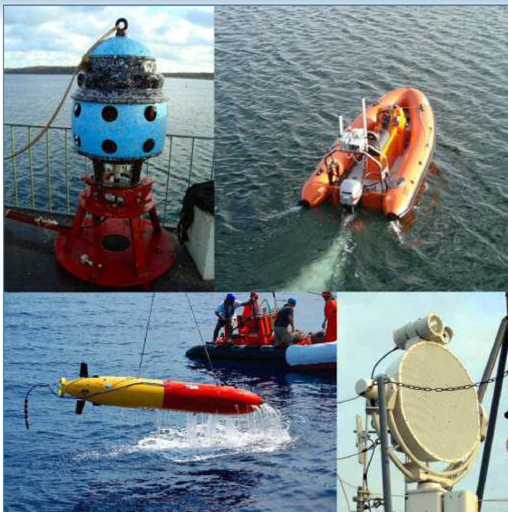
MOOS software runs on a variety of hardware platforms at NURC, including (from top-left counterclockwise): a fixed sonar diver-detection system, the Mandarina ASV, a long-range acoustic device, and the Ocean Explorer AUV.
