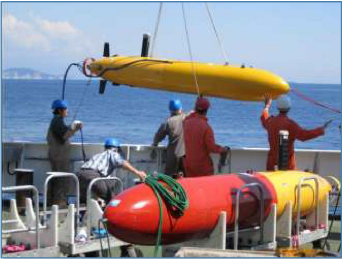
Figure 2: Two OEX AUVs outfitted with towed arrays, on-board processing and communication systems.
