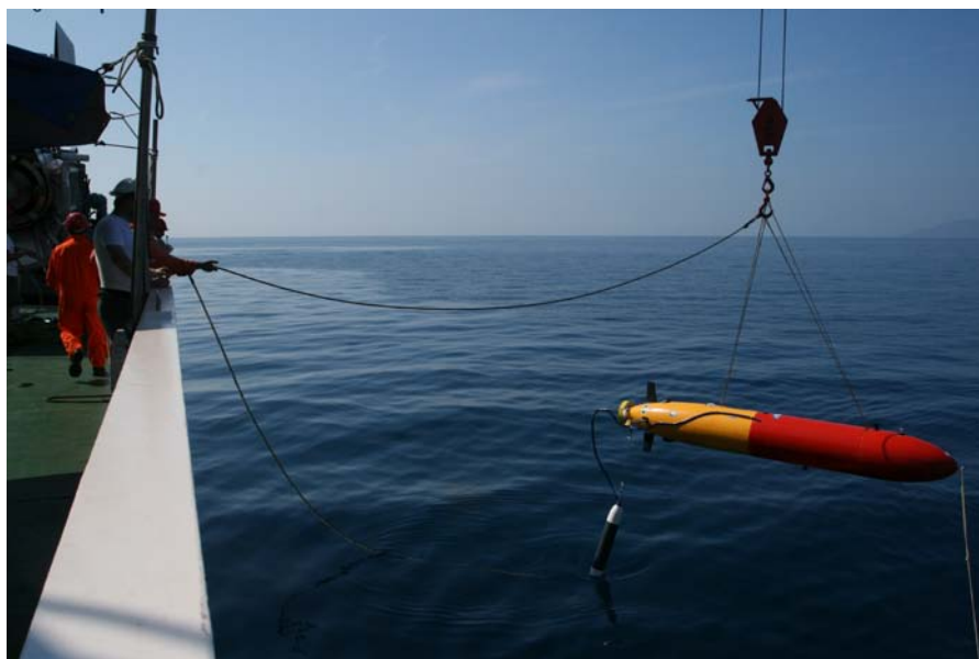
Figure 1. OEX AUV being lowered into the water the towed source can be seen dangling behind the AUV and behind, that looping through the water is the BENS towed array.
