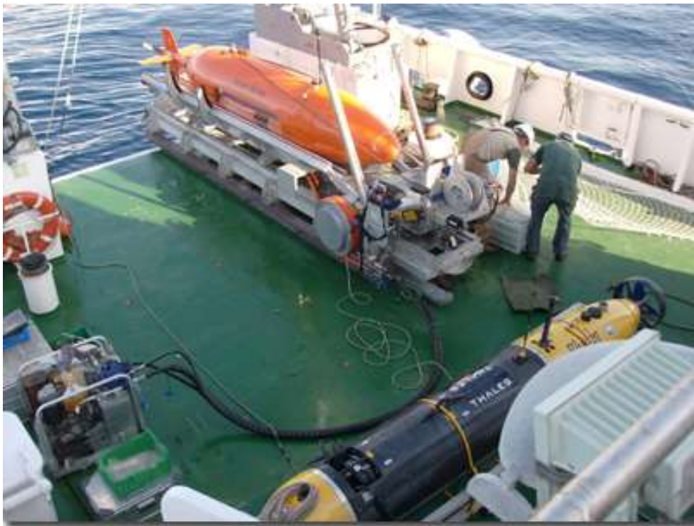
CATHARSIS 2 Trial tested two AUVs, equipped with different high-resolution SAS systems: HUGIN AUV (top) and MUSCLE AUV (bottom).
