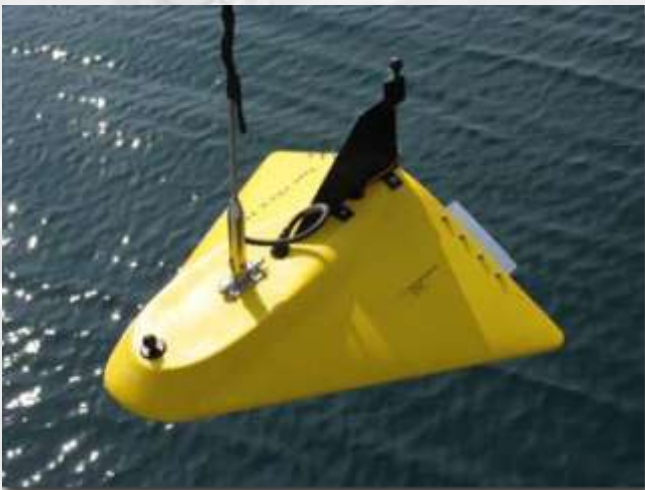
The towed CPAM array uses a unique tetrahedral arrangement of sensors to find marine mammals.
