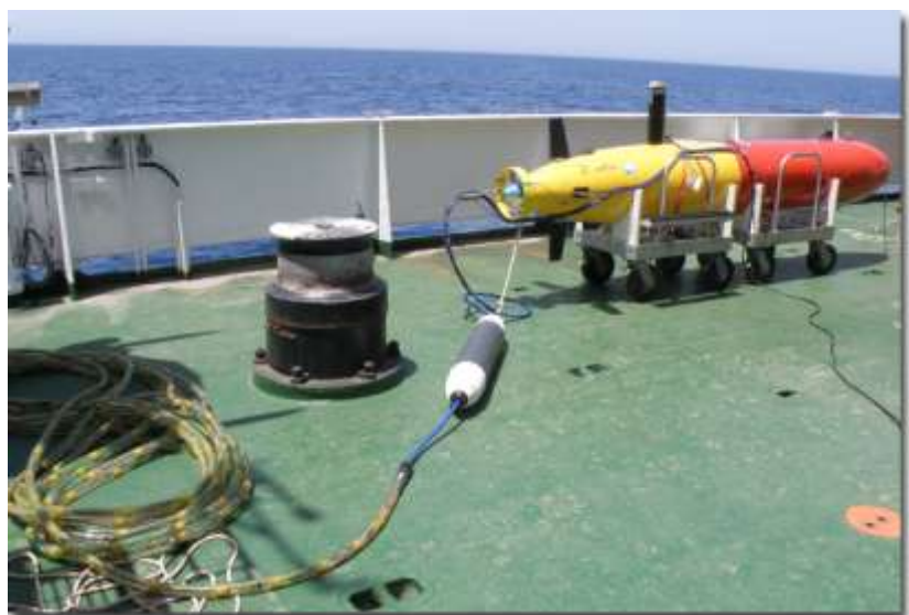
The OEX AUV set up to tow a sound source and an array, the first time an AUV has been used as a multi-static sonar platform.
