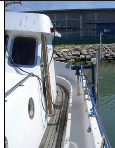
NURC scientist joined representatives from the Slovenian military, police, universities, and industry at the technical demonstrations; right, sonar mounted on side of research vessel used for pier and sea-floor inspection
