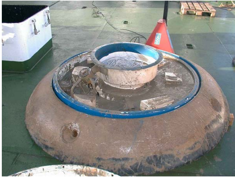
Figure 7: Barny recovered from a muddy site near the Po River outflow. Although filled with mud, it functioned normally.
