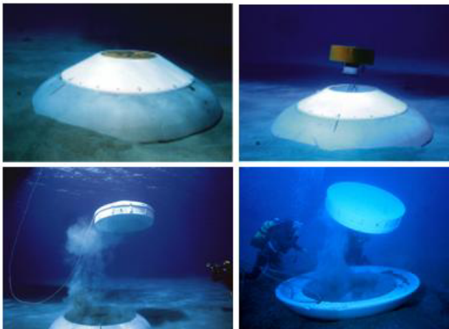
Figure 1: Upper left: Barny on the bottom in data collection mode. An ADCP looks upward from the apex. Upper right: normal recovery. Released acoustically, the circular orange float is bringing the ADCP and a recovery line to the surface. Lower left: emergency recovery. The ballast ring has been dropped and the instrument housing is rising to the surface. Lower right: emergency recovery from overturned position.
