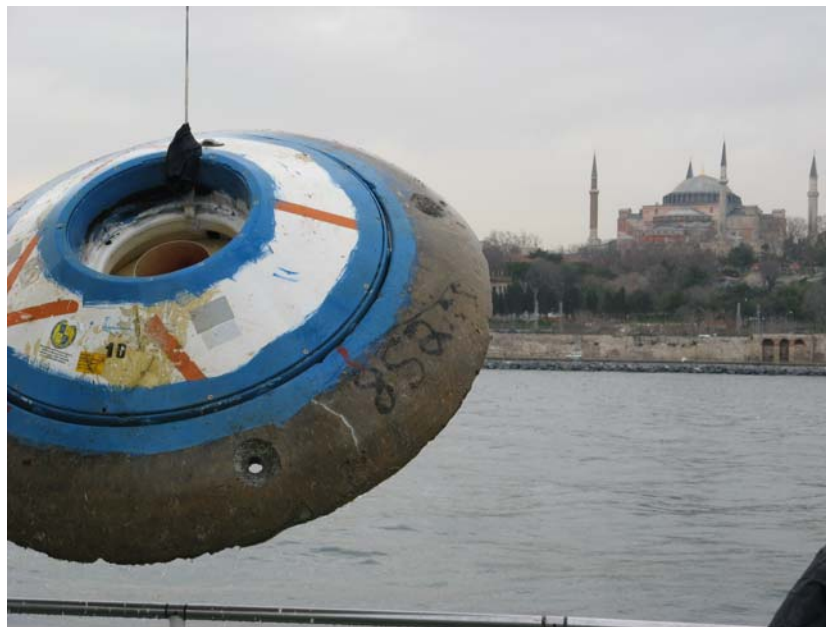
Figure 17: A much used Barny is recovered off Istanbul during a scheduled EPOS servicing operation in February 2009. Measurements will continue in the Dardanelles/Çanakkale until October, 2009.
