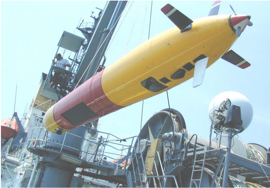
Figure EMP.3 Ocean Explorer AUV equipped with the Low frequency Synthetic Aperture Sonar which was used in the Baltic in March 2004 for a buried object detection trial.
