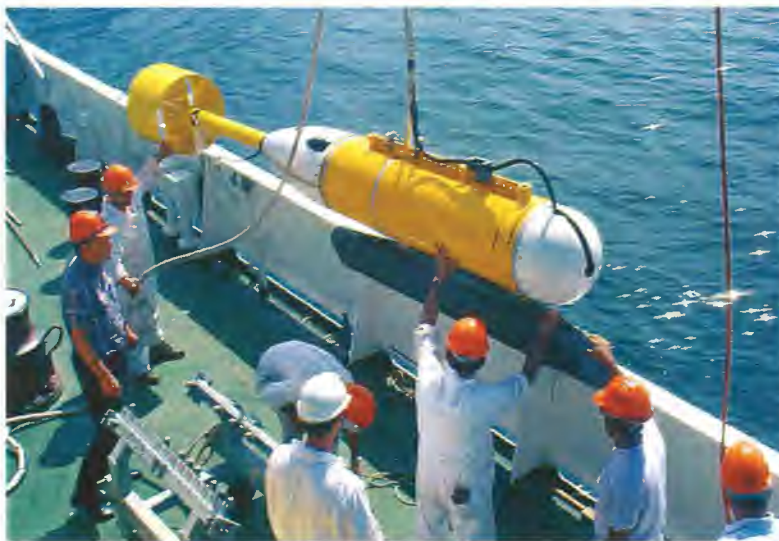
Figure 03-G.6 MASAI towbody deployed from R/V Alliance off Punta Monasteroli. The sonar is the black beam below the towbody. It operates at 100 kHz with 256 transducers spaced at 7.5 mm, for a total length of 1.92 cm. In the narrowband mode (95-105 kHz) mode, the full aperture is used, whereas in the wideband mode (90-110 kHz) only the 128 central elements are used.
