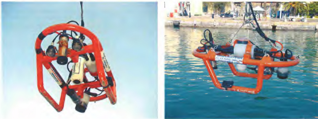
Figure 03-D.2 the High Frequency Reverberation (HFR) measurement system, shown here mounted on a sled, consists of simple and relatively small components that can be mounted on various platforms, including MILOC ships, Autonomous Underwater Vehicles (AUV's) and expendable buoys. The system transmits and receives acoustic signals from a fully calibrated high frequency transducer (80-110 kHz) and simultaneously measures its exact orientation with respect to the seafloor using an echosounder and inclinometers. Also mounted on the sled shown here are the electronics package and a small video camera. A prototype device and analysis algorithms have been developed and used as part of the MILOC exercises Rapid Response '96, '97 and '98.
