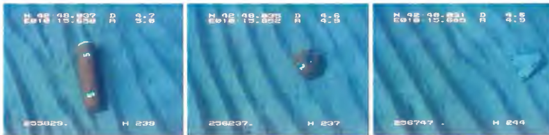
Figure 03-G.16 MP80, Manta and Rockan mines identified by means of AUV video. The AUV coordinates are displayed on the upper left corner, the AUV depth and altitude on the upper right, mission time on the lower left, heading on the lower right.
