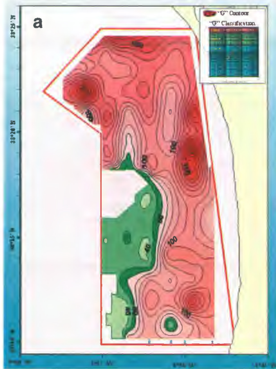
Figure 01-A.1a/b Bottom classification results (from the SACLANTCEN team embarked on HMS Roebuck) indicating low probability for impact burial of sea mines in agreement with an existing map of sediment properties.
