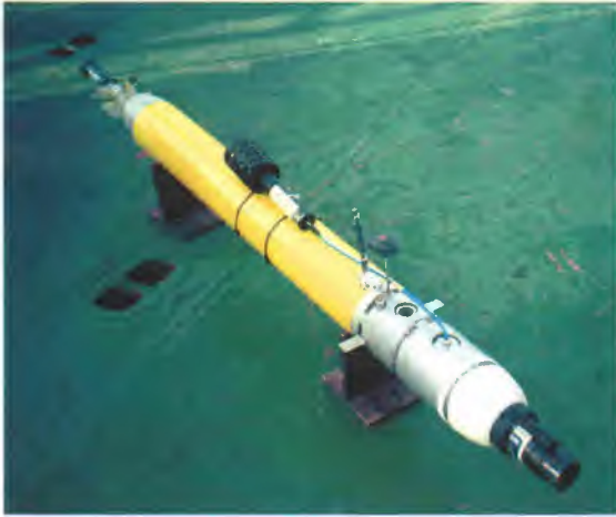
Figure 01-B.2 The TAIPAN vehicle developed by LIRMM measured salinity and temperature distribution in Biodola bay.
