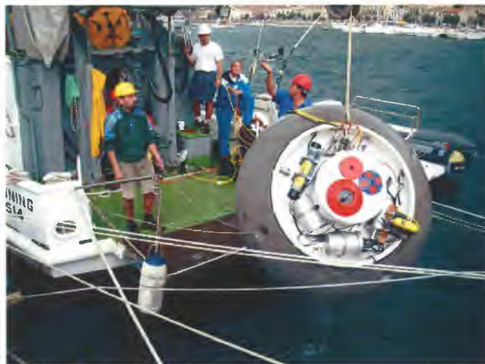
Figure 01-A.13 The SEPTR can be deployed and recovered from a small vessel. Here the cover is opened showing the interior with flotation removed. The central part is occupied by the Acoustic Current Doppler Profiler (ADCP) with 4 transducers, the water column profiler with antenna and the messenger buoy for instrument recovery.
