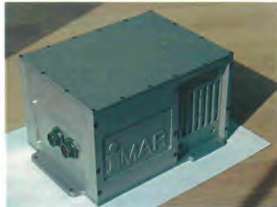
Figure 03-G.12 High grade Inertial Navigation System procured by SACLANTCEN.
