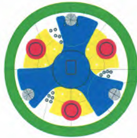
Figure 04-AB.2 Design drawing of the modifications made to the triplet attachment using plates instead of the fibre rod .
