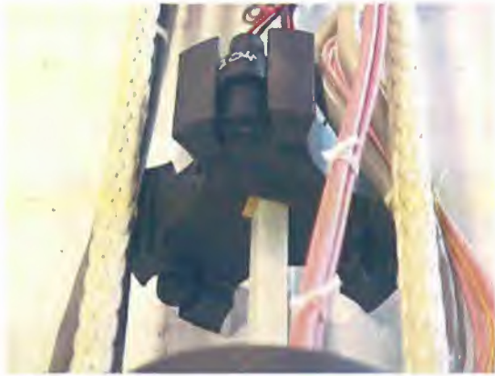
Figure 04-AB.1 Hydrophones with triplet housing attached to fibre rod .
