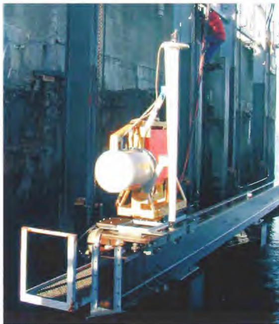
Figure 03-G.1 TOPAS parametric transmitter (orange) and 16-element vertical array (white) mounted on the chariot of the Lanvéoc rail facility of GESMA, France. Also visible is the frame and motor allowing the sonar tilt to be varied.
