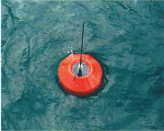
Figure 01-A.14 During operation only the profiler with antenna surfaces. Coloured differently it would be virtually invisible.
