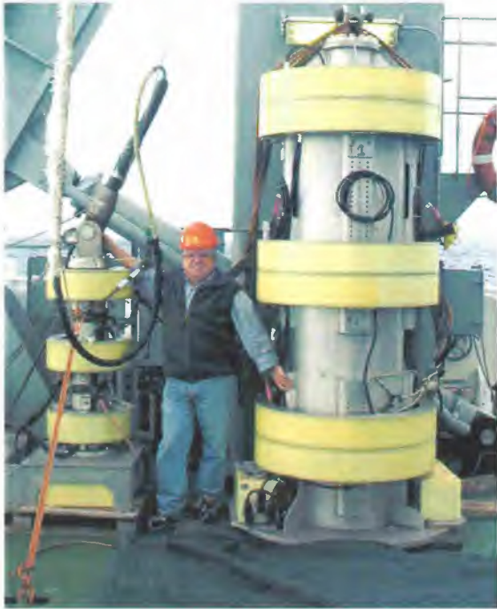
Figure 04-AB.4 High frequency (HF) and low frequency (LF) high power sound sources.
