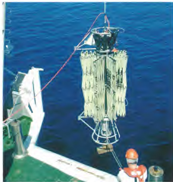
Figure 04-C.8 Deployment of the DUSS array in its retracted position.
