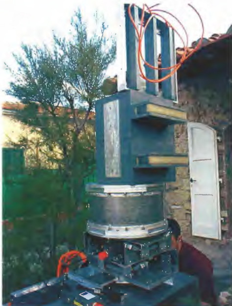
Figure 03-G.11 Multi-axis motion system and 120-180 kHz interferometric sonar (DERA, U.K.)
