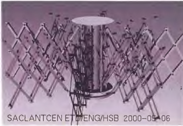
Figure 04-C.7 Showing the DUSS structure. The folding frame allows the inter-element spacing to be easily changed. Three tiers of 32 hydrophones each, arranged in a star pattern (seen to right) provide the spatial resolution required for conducting these measurements. When the arms are fully extended the total array aperture is about 4 m.
