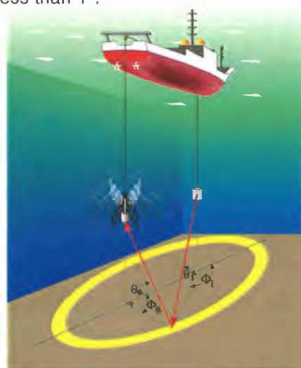
Figure 04-C.6 Showing bi-static seafloor scattering measurement geometry. The objective was to measure the dependence of the seafloor scattering strength on the four angles shown.
