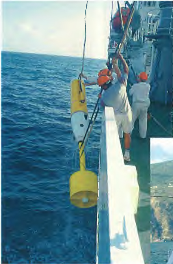
The 100 kHz programmable sonar deployed from R/V Alliance in June 99 during the MASAI'99.
