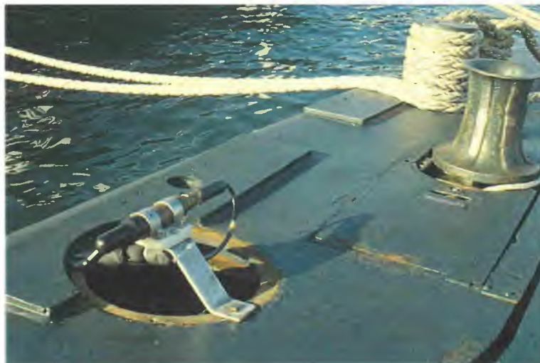
The photographs on this page show the hydrophones installed on the Italian submarine Sauro
