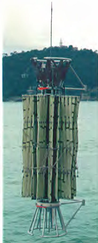
Figure 04-B.10 New DUSS prototype. deployable receiver and transmitter units.
