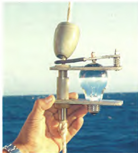
Improved version of the sound source used in project 04-C experiments
