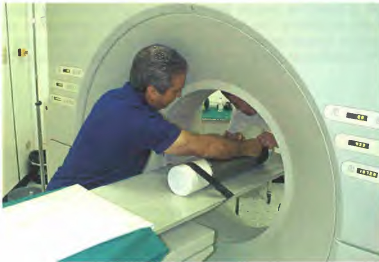
Positioning the core for the CAT scan at the Sant' Andrea hospital in La Spezia
