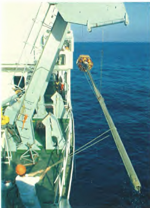
The 8 m piston corer designed and constructed at the Centre
