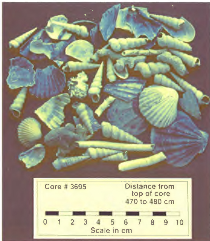
Figure 04-C.3 Shell material corresponding to high-speed layer in Figure 04-C.2 near 5 m depth sub-bottom.
