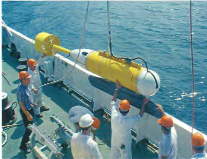
Figure 03-B.2 The 100 kHz programmable sonar deployed from R/V Alliance in June 99 during the MASAI'99.
