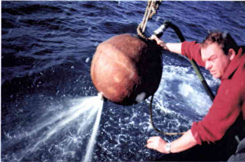
Figure 7: sphere BS1: burial method
