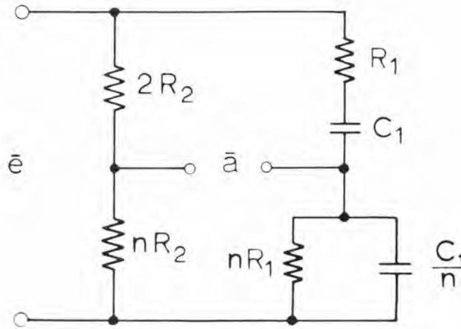
Fig. 2 Wien Bridge as Null Circuit
