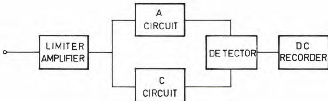
Fig. 22 Block Diagram of Sound Velocity Meter Discriminator
