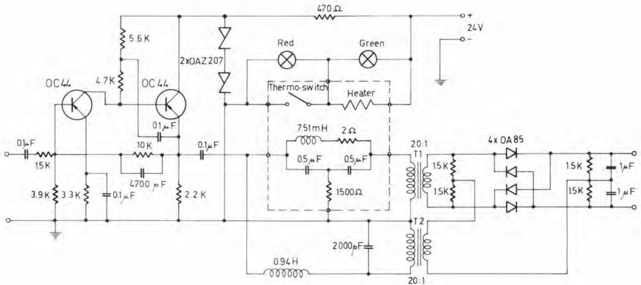
Fig. 23 Circuit Diagram of Sound Velocity Meter Discriminator
