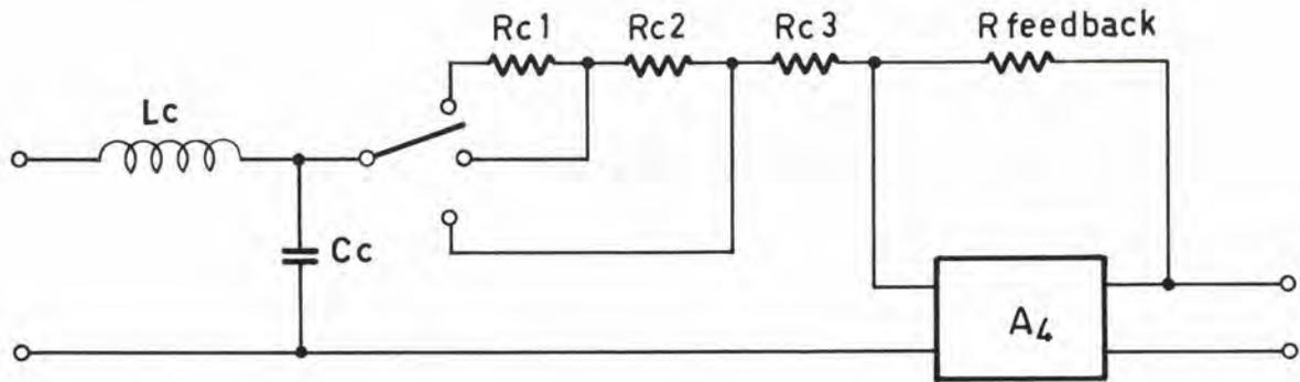
Fig. 19 Arrangement for Constant  $\left| \bar{c}_o \right|$  independent of  $Q_c$
