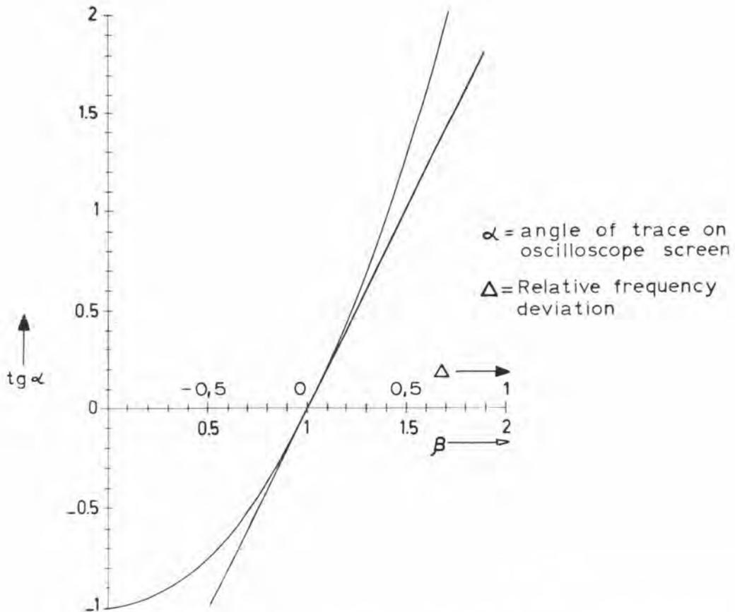
Fig. 9 Visual Display Response Curve of LC Discriminator
