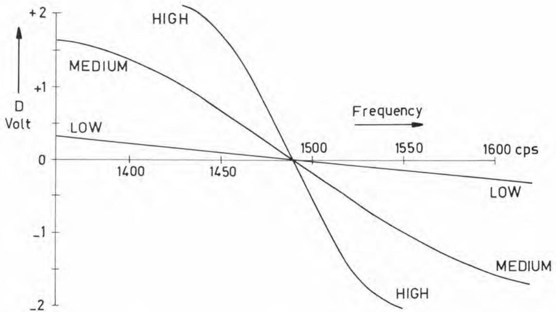
Fig. 21 Calibration Curves of Discriminator of Fig. 17
