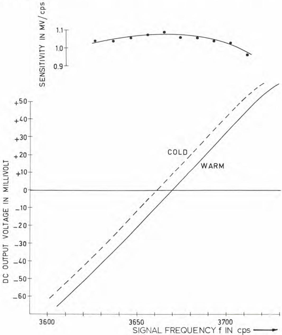
Fig. 26 Calibration Curve of Discriminator of Fig. 23
