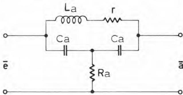
The conditions for this circuit to give an output zero at the angular frequency  $\omega_o$
