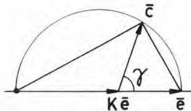
Fig. 7 Vector Diagram of the RC Phase Shifter
