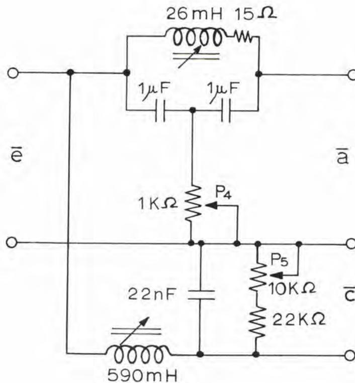
Fig. 16 Practical Circuit for LC Discriminator:  $f_o$  1.5 Kc
