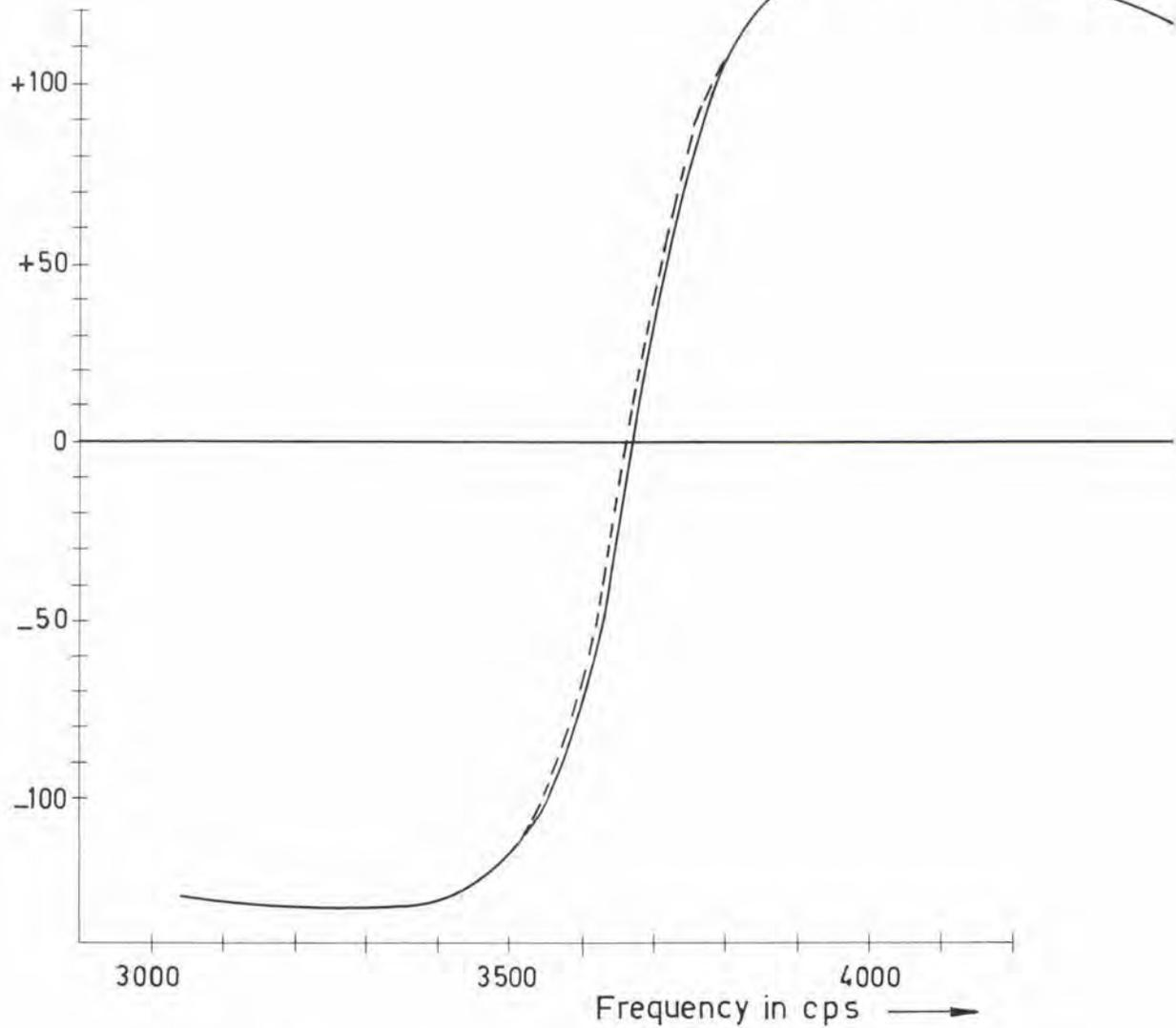
Fig. 25 Calibration Curve of Discriminator of Fig. 23
