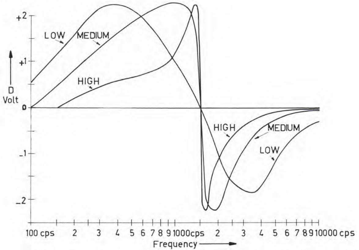
Fig. 20 Calibration Curves of Discriminator of Fig. 17
