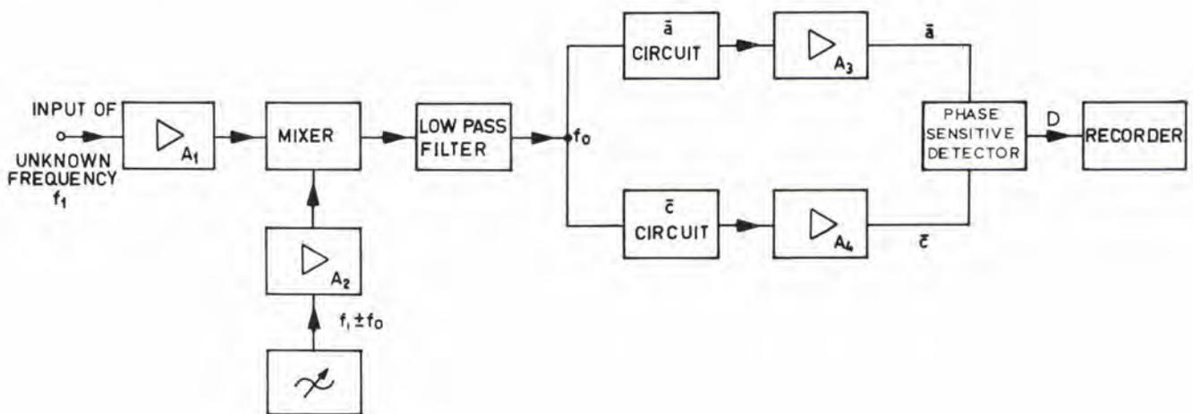
Fig. 14 Block Diagram of Complete Frequency Deviation Recorder
