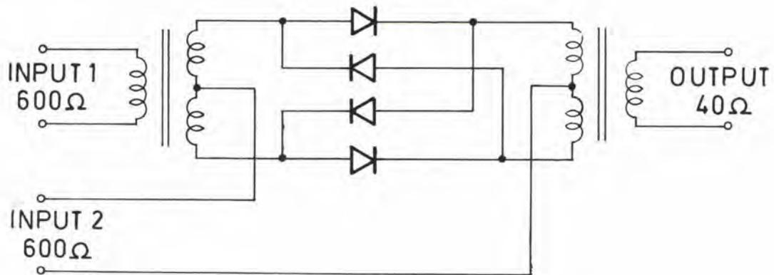
Fig. 18 "Autelco" Ring Modulator
