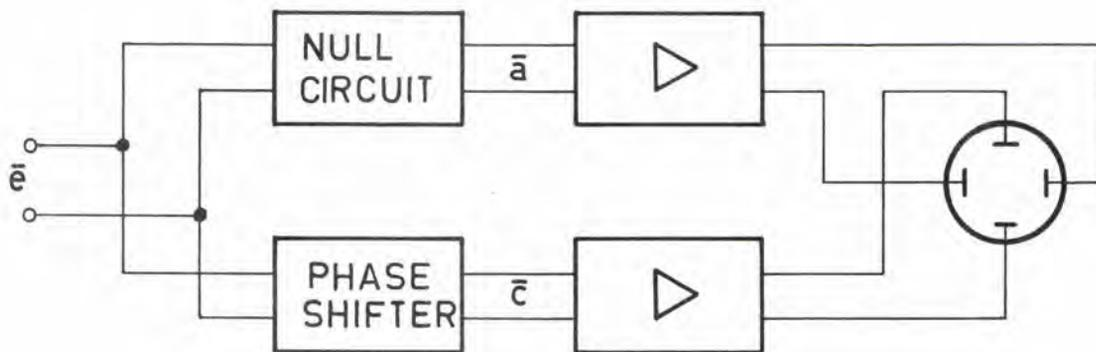
Fig. 1 Basic Block Diagram of Discriminator
