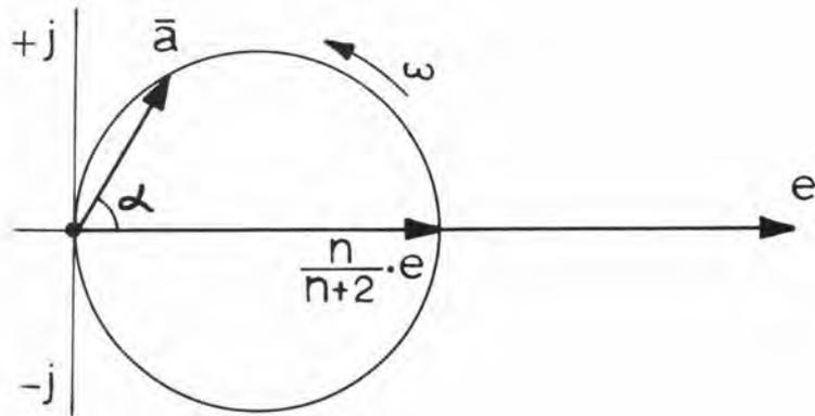
Fig. 3 Vector Diagram of the Wien Bridge
