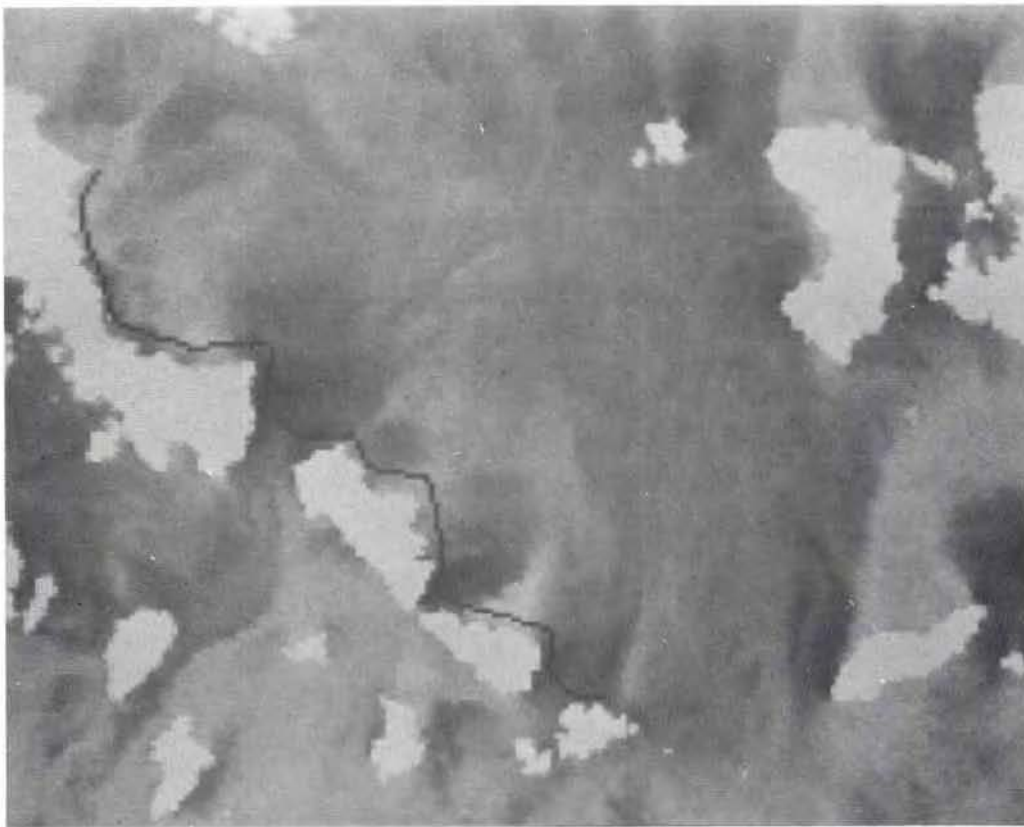
Fig. 9 Positions of the temperature and albedo profiles along the Greek islands, marked on an image of thermal IR data (Channel 4 at 11 \mu\text{m} ).
